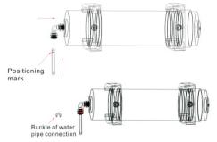
4. Insert the quick-connection elbow and water outlet pipe into the other end of the filter (water outlet).
